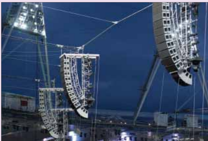
Above, left: The PA and lighting pods, designed by Jeremy Lloyd, carry the L-Acoustics PA line arrays and moving head projectors on a rigid flying frame. Above, right: the Pod on the drawing board.
