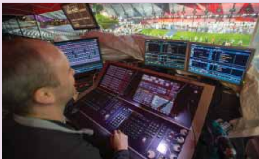
Above: An ETC Eos triggered video for the Pixel Tablets, the high level screens and the projection onto the house, via the Avolites Media Ai Infinity and Catalyst media servers respectively.
