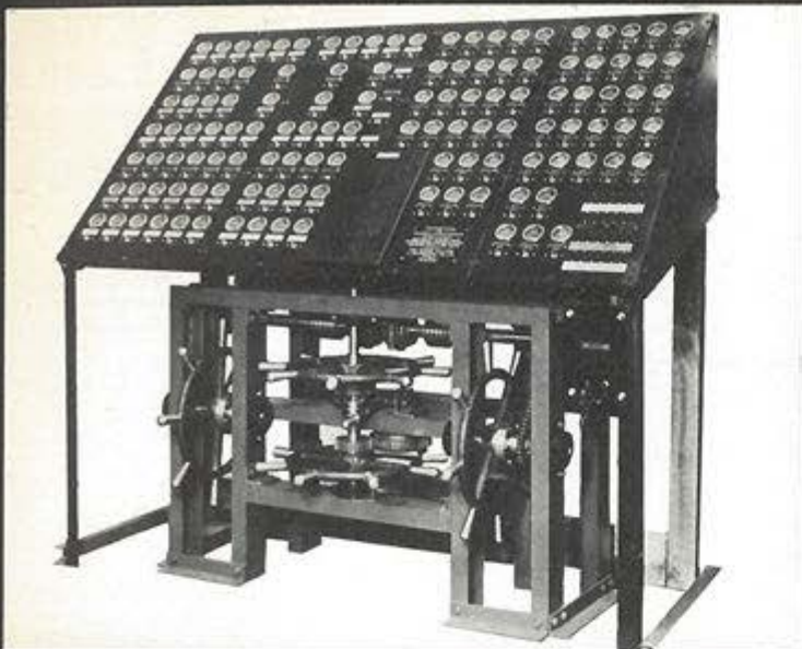
▲ The remote control panel with direct-operated capstan wheels under: Covent Garden Opera 1934-64.
