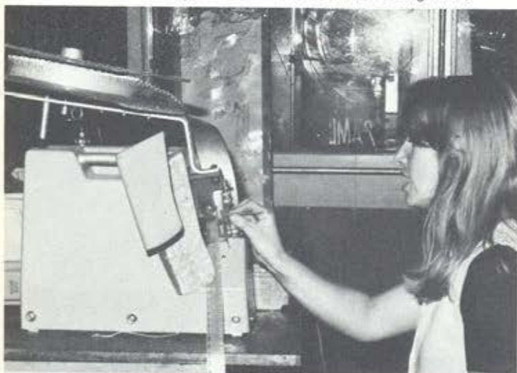
This machine automatically puts terminals onto cables.
