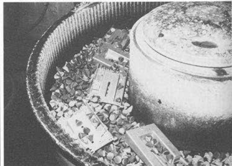
Polishing the die castings — the mystery of the plastic cones is solved!
