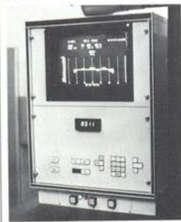
Display unit of the integrated computer system which monitors continuously the film gauge.
