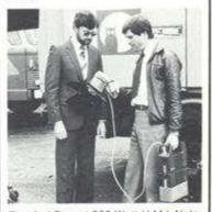
The Arri Report 200 Watt H.M.I. Note the combined buffer unit, ballast and battery pack.
