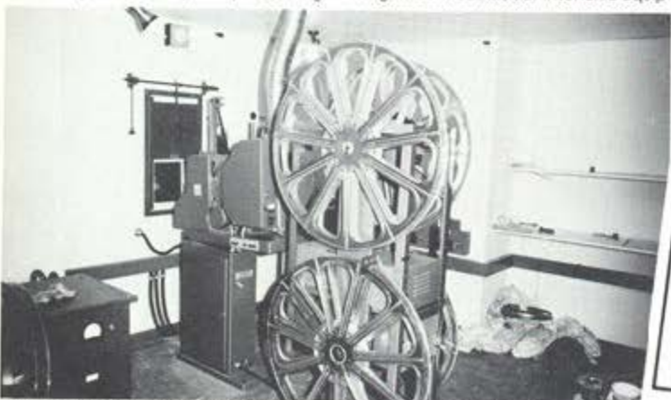
Long playing equipment. Up to six hours of continuous entertainment — courtesy of Cinemeccanica and Rank Strand Cinema.
