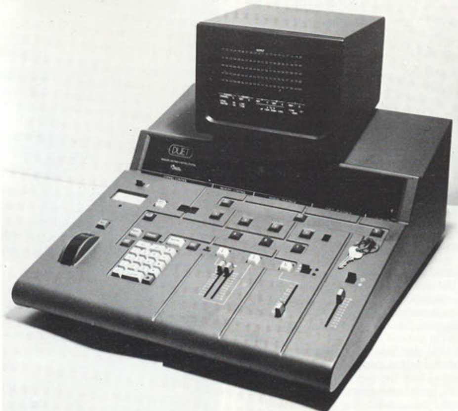
Duet console with VDU and screen close up. (Below) The mini-floppy-disc is in a similar enclosure to the VDU. Both can be located on top of the console, as illustrated, or at the sides.
