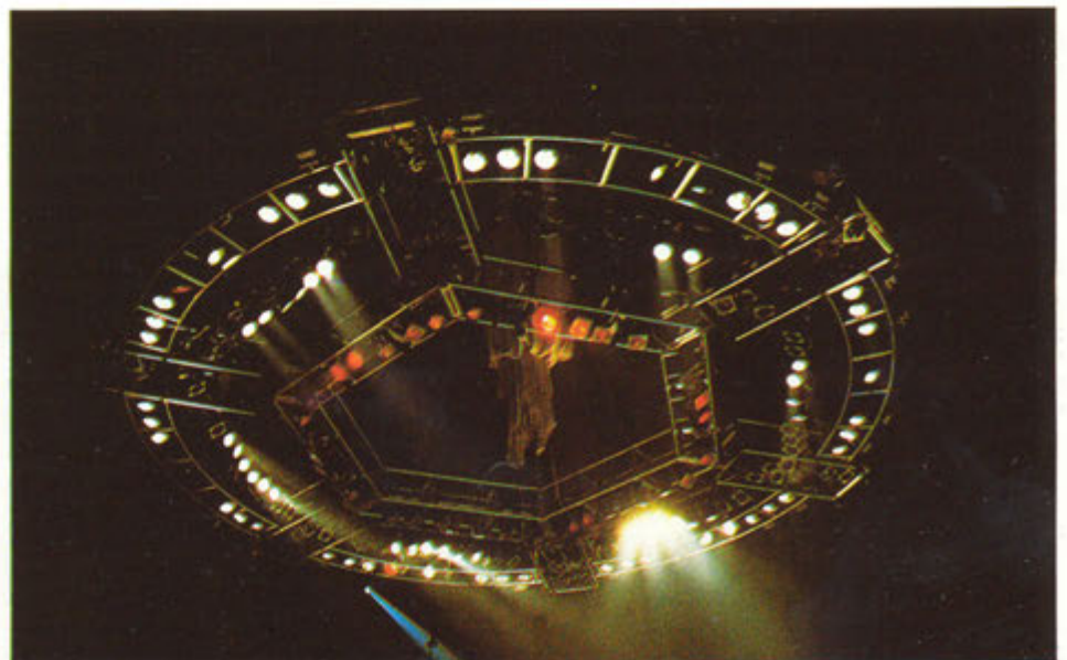
Lightweight alloy grid at Earls Court equipped with Altman PAR cans and American 120V PAR 64 lamps. Rolling Stones 1976. (Photo. courtesy T.P.A. Electro Sound)
