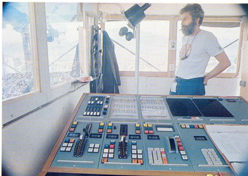
The MMS control included a pin patch enabling many special and last minute changes to be effected right up to the final run through.
