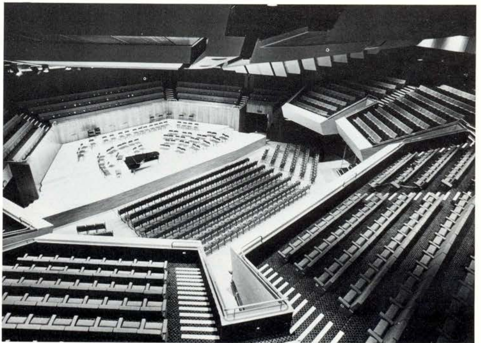
The basic form at the Hexagon is that of a concert hall. A mobile proscenium and platform lift allow for theatre and banqueting hall variations. Photo. Colin Brierley
