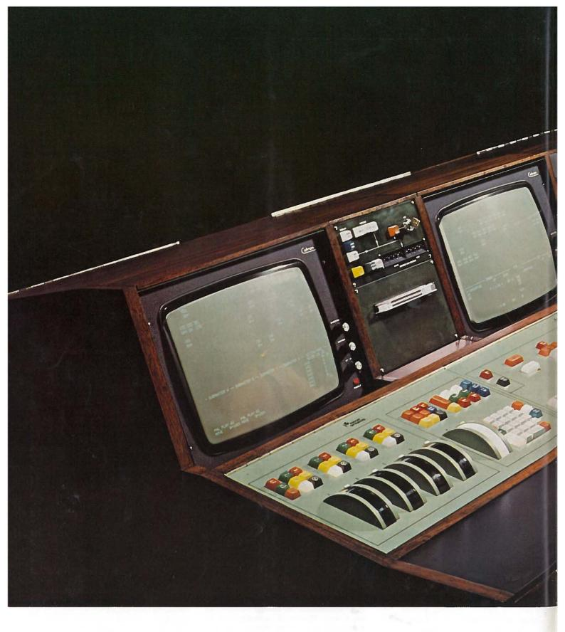
our means of access to the control of lights. This can be "played" by a skilled person with his eyes on the stage.
