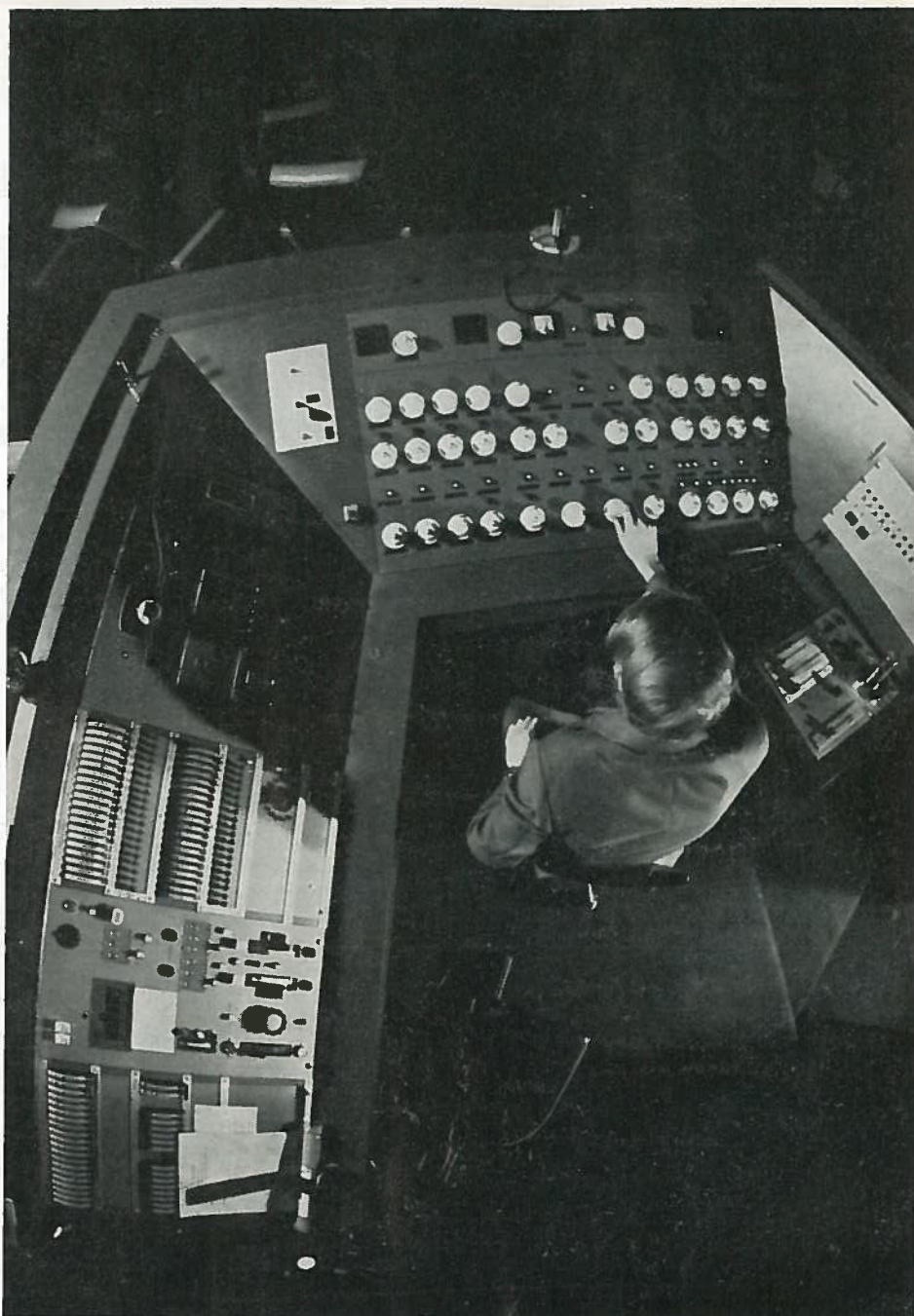
▲ Special 120-way IDM lighting control providing full level memory, also a slide change/auto start memory for each projector.
