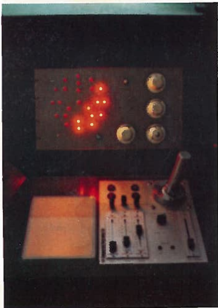
Sound can be mixed from tape, disc or microphone and patched direct to selected speakers or controlled via a joystick.
