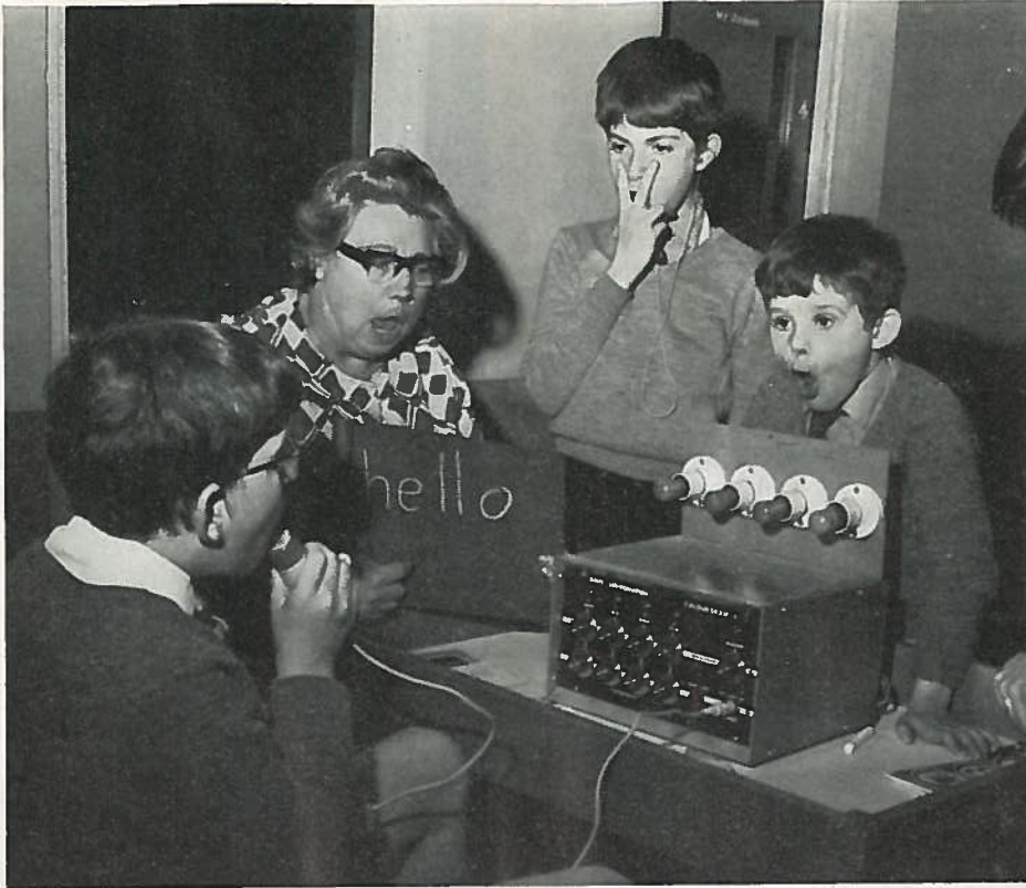
Colourgram being used for voice training by deaf children. The pupil tries to imitate the Light Pattern produced by the Teacher's voice.
