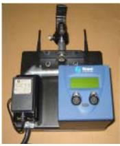
Karwat worked with Strand Lighting Canada's Richard Goode, National Sales and Marketing Manager to package a wireless, configurable and portable DMX solution. The SN110 nodes were custom mounted in an aluminum frame to hold the Access point complete with power supplies, a pipe clamp and Stage pin cord. Tom Taylor commented, "the
