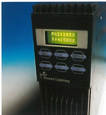
Supervisor processor module.
