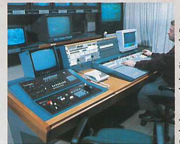
A 'twin' control room suite at RAI, showing an M24 and Gemini 2+ side by side controlling the lighting in two separate studios.
