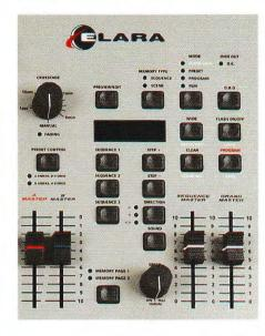
The Elara™ has a "live style" of memory control where memories are recorded onto submasters. The desk has two pages of 24 memories which, in run mode, are replayed using the preset faders as submasters. All 24 memories can be replayed simultaneously allowing complex memory mixing to be done "on the fly". Page overlay allows access to all 48 memories and the desk has comprehensive memory editing facilities.
