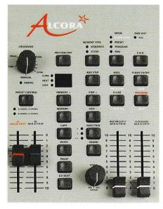
Memories are replayed sequentially using the "Go Next" button. Fades between memories and chase steps are dipless and timed. Crossfades can be stopped using the "Pause" button and memories can also be replayed out of sequence if required. The built-in effects package includes an advanced Sound chase. There is also a memory preview facility and provision for a remote 'Go' button which can be used if your budget doesn't run to a lighting operator.
