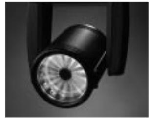
The small, lightweight VARI\*LITE® VL5B™ wash luminaire uses a 3200°K tungsten halogen lamp and cold mirror reflector that removes heat from the light beam, eliminates fans and associated fan noise, and reduces heat on stage.
