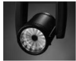
The compact, lightweight VARI\*LITE® VL5™ wash luminaire uses a 3200°K tungsten halogen lamp and cold mirror reflector that removes heat from the light beam, eliminates fans and associated fan noise, and reduces heat on stage.
