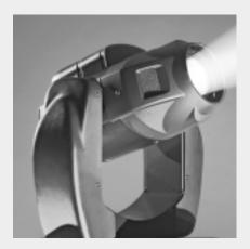
The VARI\*LITE<sub>®</sub> VL2201<sup>™</sup> spot luminaire is based on the VL6B™ spot luminaire. The VL2201 luminaire features an upper enclosure that houses the control electronics as well as a power factor corrected arc power supply for the Philips MSR400SA arc lamp. The VL2201 luminaire also features a zoom optics system and rotating gobos. The luminaire is small, lightweight, and virtually silent.
