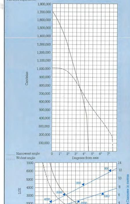
The figures on the diagonal lines indicate the illumination value in lux at beam centre.
