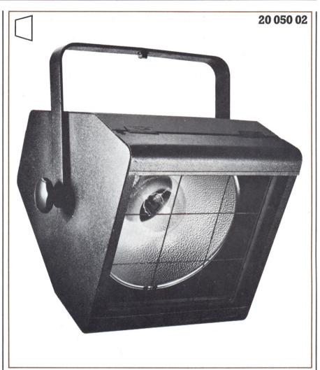
General-purpose theatrical Floodlight with a symmetrical, wide angle distribution suitable for small scale cyclorama lighting if spaced at least 2.5m from the cloth or wall; also for close range illumination of door and window backings.
