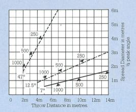
The figures on the diagonal lines indicate the illumination value in lux at beam centre.
