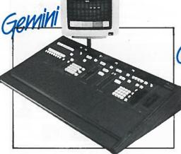
The newest memory lighting control for theatres, clubs and touring companies, Gemini offers 180 channels of multiplexed control, electronically patchable to expand the system for up to 384 dimmers. Features include twin playbacks, submasters, disc library storage, 80 group electronic back-up, colour VDU, remote controls and an advanced programmable effects system.
