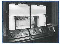
HE highly acclaimed M24, designed for the smaller lighting rigs, owes so much to its heritage. From IDM came the concept of recording from an associated fader wing, from MMS the wheel and keypad control, from Lightboard the multipart fades, and from Galaxy the speed of operation. Although small in size, the power of the 60 channel (now 120 channel) 'baby' of the range has been internationally adopted in professional and amateur theatre, TV and hire companies.
