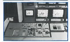
MS (Modular Memory System) was the first mass produced memory control and jumped two hurdles in a single stride: it took full advantage of low-priced integrated circuit technology, and dispensed with a rocker switch per channel in favour of a calculator keypad and wheel, to control up to 480 channels. A range of user selectable modules gave theatres and TV studios in 30 countries the chance to light with a custom-designed control at an affordable price.
