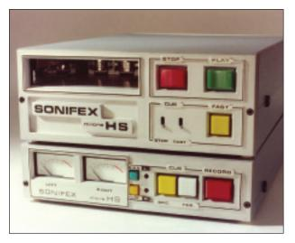
machine, and erasing carts quickly required yet another machine, the bulk cart eraser. Playback required regular head cleaning and alignment to ensure the best playback quality. And carts themselves were relatively expensive and, with their convoluted tape path and special lubricated tape, not terribly long-lived - long-running shows could outlast their sound effects carts!
