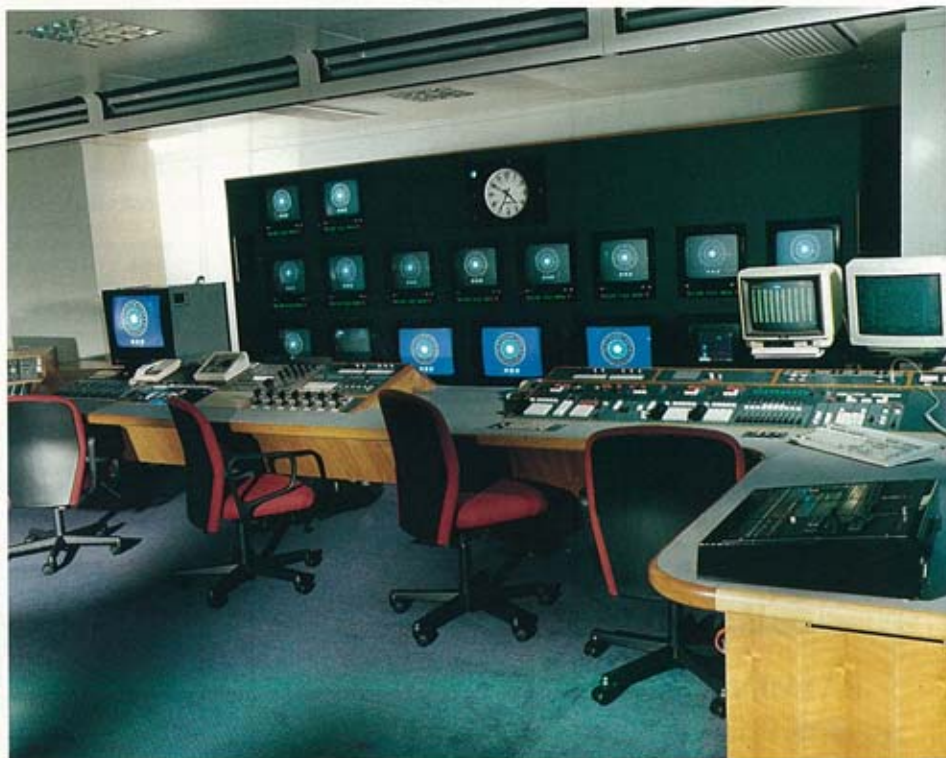
The lighting and vision control room in TC6: the Galaxy console is at the right with the channel mimic and BBC studio mimic monitors above and optional Pulsar effects control on the side desk. The lighting director sits at the central position with vision balance operator and system engineer at his left.
