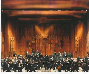
stage canopy two metres and suspending an array of the curved acoustic reflectors ascending steeply from the stage to the main body of the hall, full-bodied sound is distributed more consistently to all parts of the auditorium. The acoustic is equally adjustable for the more intimate requirements of recitals or chamber concerts, right up to the full scale requirements of a symphony orchestra and chorus.
