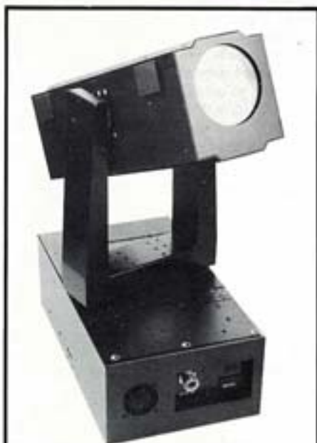
The 400 watt HTI Strand Lightscan is a hard-edged automated fixture with two internal 16-colour changers, five gobos, remote control of iris, dower and focus, variable speed, and high digital accuracy. Meteorites will soon hold a considerable stock of these powerful light sources - ideal for major concerts or industrials.
