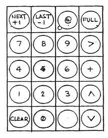
(NEXT +1) BUTTON -- The NEXT or +1 button allows the operator to step in ascending order through a series of memories, channels, dimmers, or effect steps as displayed in the LED windows.
