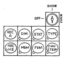
(REC A) BUTTON -- Depressing the REC A button after selecting a memory number will record the current channel readings of Scene A into the selected memory.
