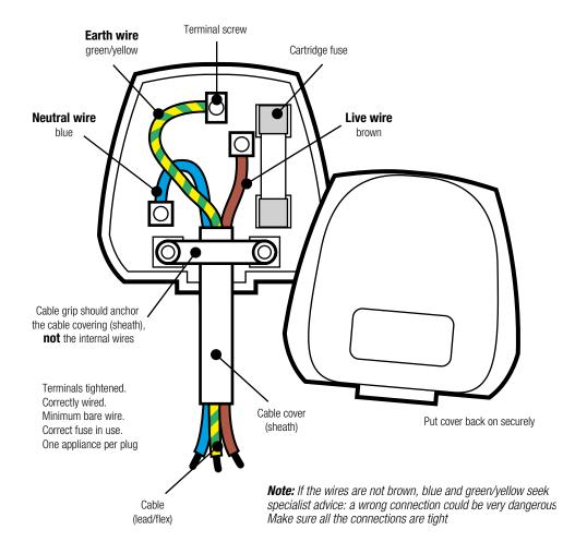
If a lead or plug is damaged, replace it with a new one or repair it.
