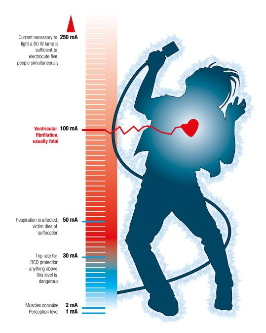
Figure 1 Relative magnitude and effect of electric current
