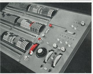
14. To pile two cues: Select the two cues required and read as above, but use both C and D faders in any relationship required. Under these circumstances, the white lamp display in the dimmer lever scales comes from two piled sources. Should it be necessary to know what each is doing, the display of one can be extinguished for the time being by pushing the tab between the two faders towards the other.
