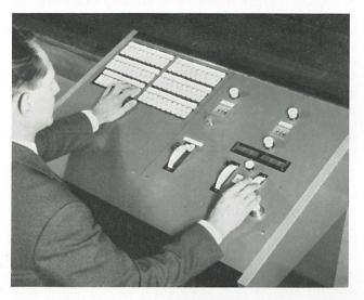
rehearsal. A lighting control is tested to the full at rehearsal, and Strand System IDM is designed to cope with these conditions of strain, speed, and indecision in comparison with which the rest is simple. Absence of delay and the ability to modify—to change one's mind—these are the two great requirements. It is speed plus the need to skip backwards and forwards as rapidly as memory itself that spell the doom of punched card, adjustable plattens, tape, and all the rest.
