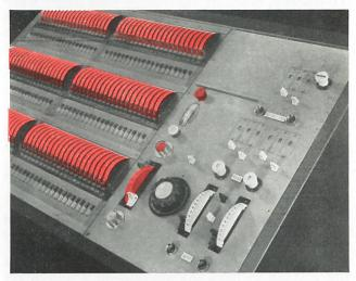
2. To fade in or out all lighting: Use Master A in conjunction with individual dimmer levers in the normal manner. Masters are all-electric and do not move the individual levers.
