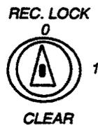
The keyswitch acts as a 'Record Lock' for the disc system. It is also used, together with the DISC CLEAR key underneath., to initiate a 'disc clear' operation.
