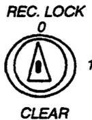
The keyswitch acts as a Record Lock when the system is in use. When the switch is in the '0' position, the Record keys are inoperative.
