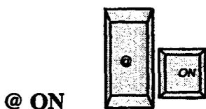
If pressing the ON key is immediately preceded by operation of the '@' key, the selected channel will be set ON at the level currently saved in the 'ON' store for that channel. This is irrespective of the illumination of the 'ON' key. The level stored for the channel in the ON store will not be changed.
