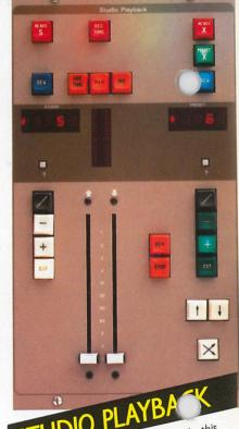
The recorded lighting states are recalled by this control panel, from where the change to the current studio lighting is made either manually or current studio.
