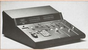
However, as an alternative to even a simple above-zero LED mimic, there is a free-standing Visual Display Unit providing alpha-numeric mimic of the percentage intensity of every control channel and the content and state of all master functions.
