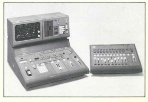
If submastering is required a free standing desk is available with 10 submaster stores, each with a group fader with 50% overrun capability. The DUET 2 memory can be used to record and recall the allocation of channels to particular submaster
