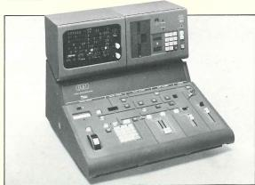
The Floppy Disc Unit is one optional peripheral unit; like the VDU it is free-standing and need not be sited on top of the console. It can be used to supplement the fast-access memory of the DUET 2 but is especially useful for repertoire library storage. For a hard copy a desk top Printout Unit is available to list the recorded level of every channel for each DUET 2 console memory, plus recorded fade time and any recorded link sequence.
