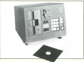
The momentary action keyswitch initiates a complete Clear of a disc and also the essential formatting of a brand new disc to suit the number of control channels. During a transfer the top numerical indicator changes to show the Memory number currently being transferred.
