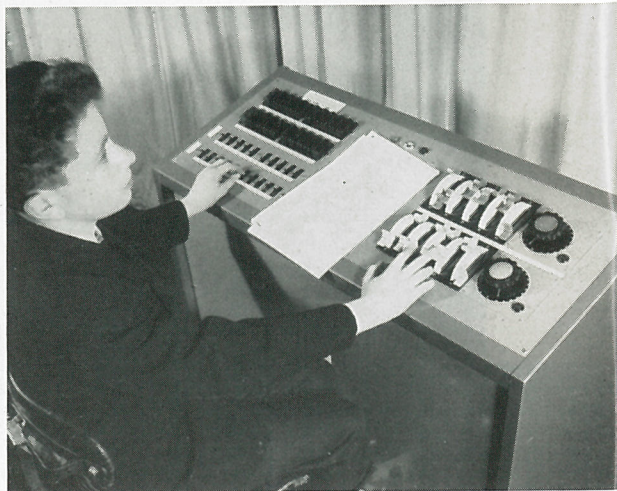
20-channel 10-dimmer Strand Ten/20 control. Example of presetting made possible by the new thyristor dimmer. All dimmers are variable load and everything including the socket outlets is contained within the portable console.
