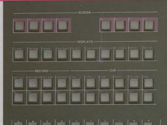
The Screen, Record, and Cue key pads are your fingertip controls for the flexibility of the Prestige 3000. The eight Screen Keys are soft keys whose functions are unique and tailored to each of the ten displays. Each of these independent controls is clearly labeled at the bottom of the selected display. Soft keys save clutter on the board since only the keys you need for the work you are doing are present. You'll work faster and more accurately.
