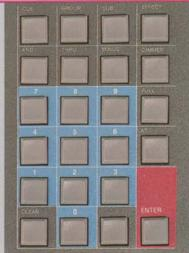
The Control Keypad is used to write out and enter commands for the Prestige 3000. You can prepare channel lists, specify output levels and enter numeric data. In addition, this control group lets the operator add to a channel or dimmer list and remove items from those lists. The user can also create subsets of channels, groups or existing cues to be
