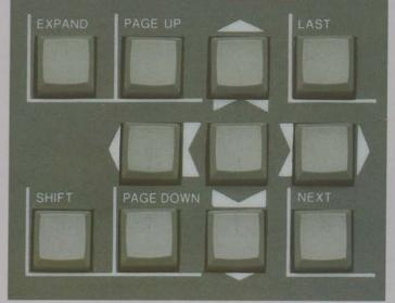
Reviewing your screens or paging through the Prestige 3000's monitors is fast and simple. The Position Keypad makes it effortless to move up, down, right and left through the system's displays. It lets you instantly leaf through multi-page displays at the push of a button and step sequentially through lists and dimmer setups during dimmer checks.
