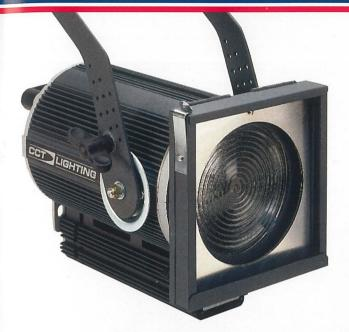
The Freble lamphouse contains a lead screw for adjustment of focus of the lamp (fitted base down) and by releasing the safety screw and loosening the locking knob the Fresnel or Pebble lenses, with their different sized front lens holders, may be fitted onto the lamphouse.
