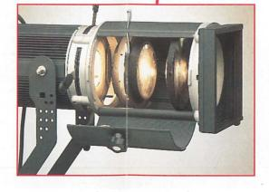
A full width access door in the fully rotating lens tube allows the operator to carry out maintenance and cleaning of the lenses, whilst the structural integrity of the tube is preserved by the cunning design of the castings, extruded profiles and their integral hinge system.
