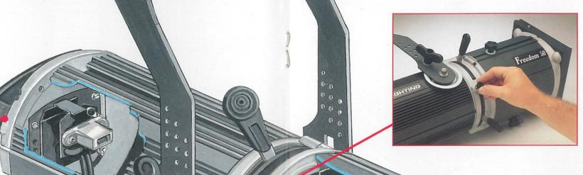
The bayonet fittings that mate the lens tube to the lamphouse have a safety screw and locking knob. By aligning the indicator on the lamphouse with the raised line on the lens tube the two may be parted provided the safety screw has first been released. When the locking knob is released the lens tube may be rotated through 360°.
