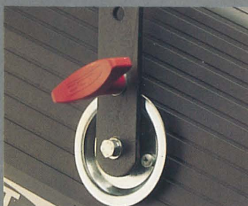
Locking Knob and Yoke height adjustment.
