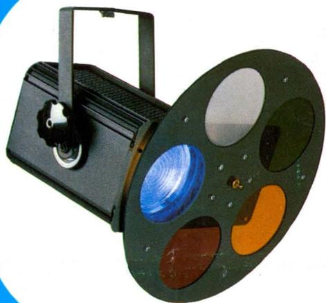
Remote control 24V AC Chromatic Wheel system with five colours and continuous selection. Standard controls for up to ten units in any combination of two, four or six groups operating on ring of three 0.5mm<sup>2</sup> control cables. ColorPad Matrix with status feedback. Wheel and Semaphore systems are available for other CCT luminaires.
