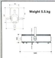
Typical performance based on Calibrated:- T27 650W, 240V, C13D biplane 400Hr, 3100K, 14,500 Lumen
