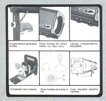
The Minuette Range is a complete family of luminaires with individual but complementary optical and photometric characteristics designed around 500 and 650 Watt tungsten halogen lamps. Construction is in general of finned aluminium extrusions formed aluminium and sheet steel. Spot lights are fitted with a full width heat insulated rear handle and external 3 conductor cables are one metre long 1.5mm<sup>2</sup> high temperature silicone.
