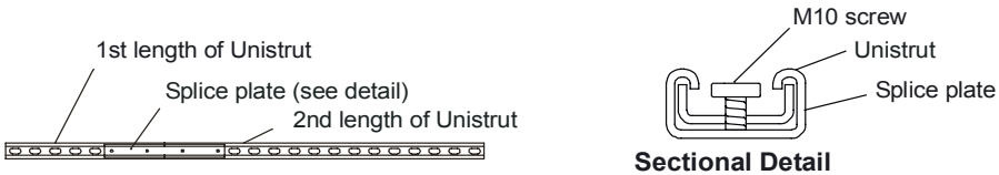
Figure 2-2 Construct Unistrut crosspieces
