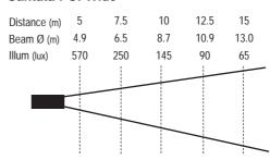
To calculate lux levels at any throw distance divide the following factors by the distance squared:
