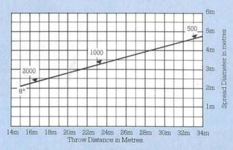
The figures on the diagonal line indicate the illumination value in lux at 2° offset
