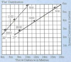
The figures on the diagonal lines indicate the illumination value in lux at beam centre.
