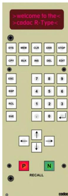
FIG 6-4. R-Type Central Control Module (lower section)
