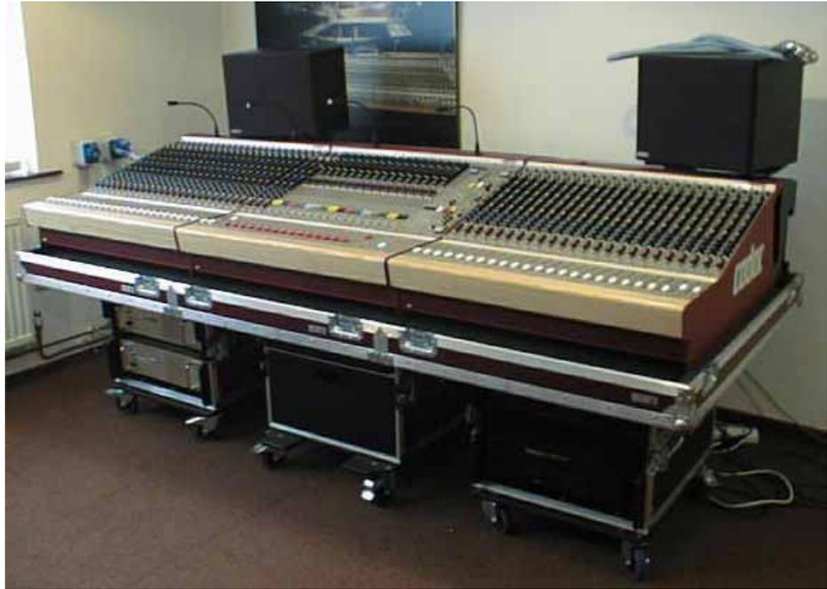
FIG 3-9. Frames ready for cabling together
