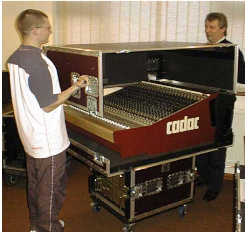
FIG 3-7. Removing the case lid.
