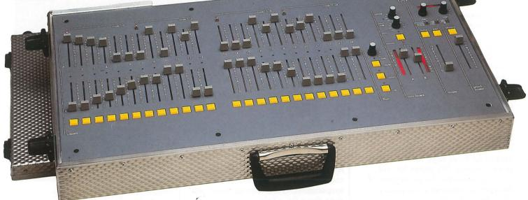
The FX Control Systems may be supplied either in lightweight rigidised aluminium flightcases, for location and rental work, or in smart, ergonomically designed consoles, for permanent installation in smaller studios and theatres. Whether you choose FX12, FX24 or FX36 (at 12, 24 and 36 channels respectively), the specification is the same.
