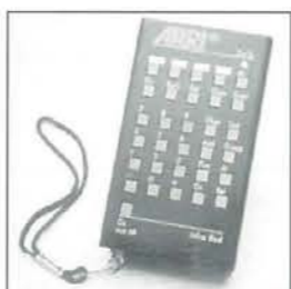
Infra Red Handset Handheld remote works with cable or infra red receivers at up to 40m range
