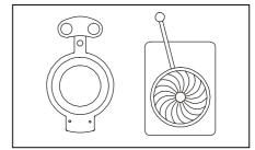
To mount the accessory in the aperture slot ensure the pattern spring clip is facing to the front of the luminaire and slide into the slots formed as part of the shutter plates.
