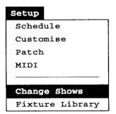
When the WHOLEHOG is turned on, it automatically opens the last show used. Use Change Shows to load, archive, or restore shows. The show currently loaded on the desk is listed after "Current Show"
