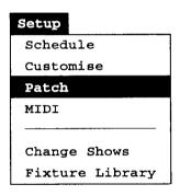
Now that you've told the desk how many of each fixture type you're using, select the Patch window to set up each fixture's DMX address.
