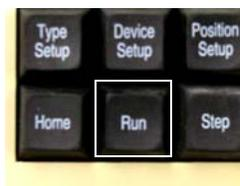
Figure 91-Run Key Moving Lights Keypad
